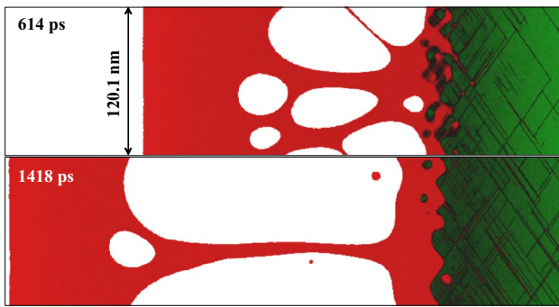
Fig. 1 Maps of central symmetry parameter showing local order in ion subsystem in MD simulation with the absorbed fluence F_{\text{abs}} = 136.9 \text{ mJ/cm}^2 , see run 3 in Table 1. Red colors correspond to molten gold, green to solid. F_{\text{abs}}/F_{\text{abs|abl}} = 1.16 , v_{\text{surf}}^\infty = 130 \text{ m/s} , T_{\text{spall}}^\infty = 1.7 \text{ kK} , d_{\text{spall}} = 80.3 \text{ nm} . Here F_{\text{abs|abl}} is a thermomechanical ablation threshold, which is equal to 118 \text{ mJ/cm}^2 according our simulations
