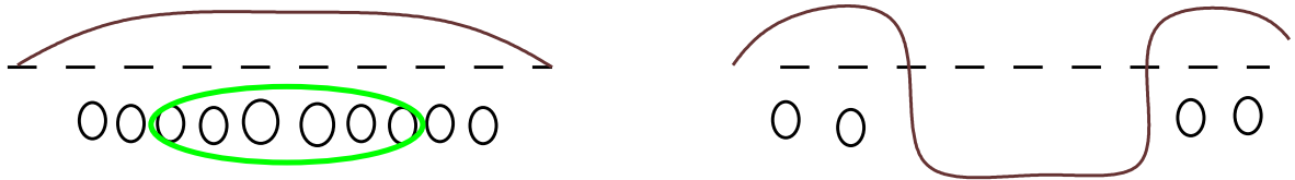
Fig. 4. Process of cavitation and spallation: multiple nucleation in the elongated horizontal layer under the spallation shell d_{spall}(y) shown in Fig. 3 (left); merging of small bubbles in the central region into the large void shown by oblate ellipsoid (left); run-away of the spallation shell d_{spall}(y) and formation of the crater with sharp lateral walls (right); the walls correspond to the circle r = y_{abl} where fluence achieves threshold F_c \exp(-y_{abl}^2 / R_L^2) = F_{abl} (right); dashed line is an initial boundary.
