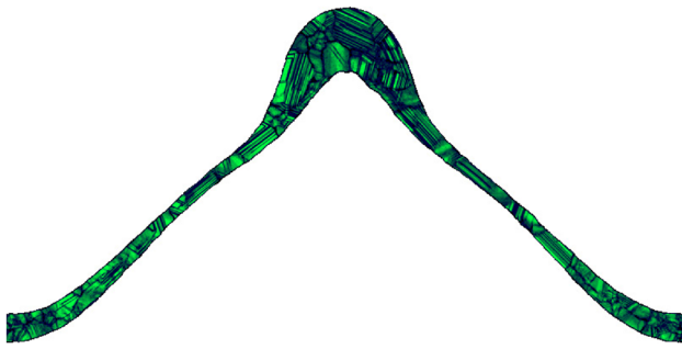
Fig. 7 Local atomic order parameter mapped in the final cross section of axial-symmetric solid bump for the non-ejecting run 30 is listed in Table 2 and Fig. 6. This view is often met in experiments at the intermediate pulse energies, see, e.g., [14] or Fig. No. 3 in [26]. Let us pay attention to the grains of the nanocrystallites forming the bulged shell. The dark lines show lattice defects such as dislocations or boundaries between grains. The horizontal size of cross section is L_b = 270 nm
