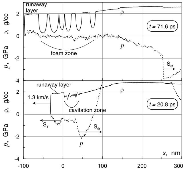
**Fig. 4** Formation of a runaway layer on the left end of cavitation zone at 20.8 ps, and detachment of the runaway layer associated with decay of dynamically weak foam at 71.6 ps
