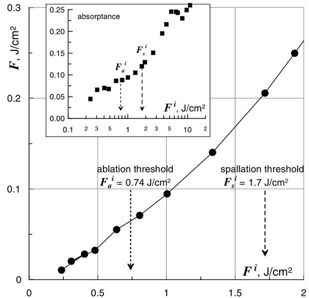
**Fig. 7** Ablation and spallation thresholds, and the experimental absorptance  $A(F^i)$  and absorbed fluence  $F(F^i)$
