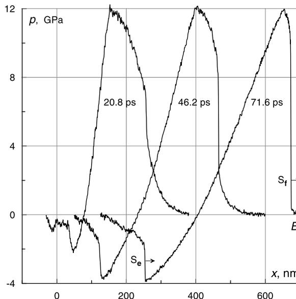
**Fig. 3** The end of acoustic decay: the twofold pulse moves from the front boundary. In continuation of Fig. 2
