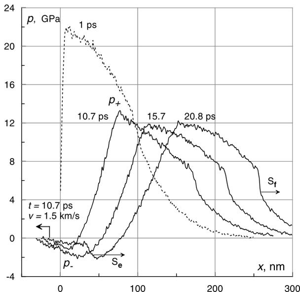
**Fig. 2** The process of acoustic decay. The initial pressure  $p(x, t = 1 \text{ ps})$ , and formation of quasi-steady twofold pulse with two shocks  $S_e$  and  $S_f$
