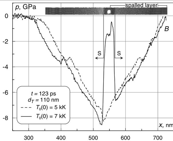
**Fig. 6** Pressures for the rear-side spallation below threshold ( $T_0 = 5$  kK), and above threshold ( $T_0 = 7$  kK) with density map for  $T_0 = 7$  kK. The profiles are similar except the zone around the rupture where pressure spike grows fast
