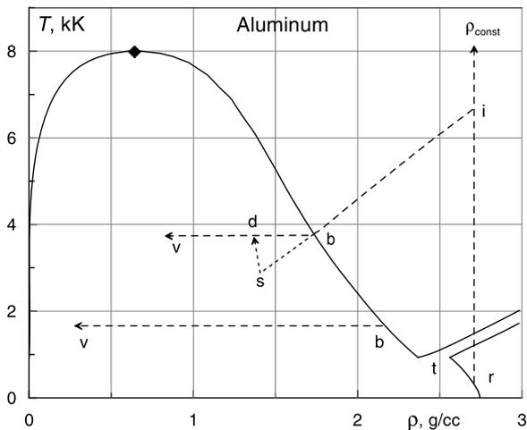
**Fig. 1** Phase path  $r-i-b-s-d-v$  of an Al particle of target irradiated by fsP. Phase diagram taken from [10]
