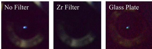
FIG. 2. Acquired optical images of the SXRL pulse irradiating the LiF surface by the CMOS detector without a filter, with a  $0.2\ \mu\text{m}$  thick Zr filter and with a  $100\ \mu\text{m}$  thick glass plate.
