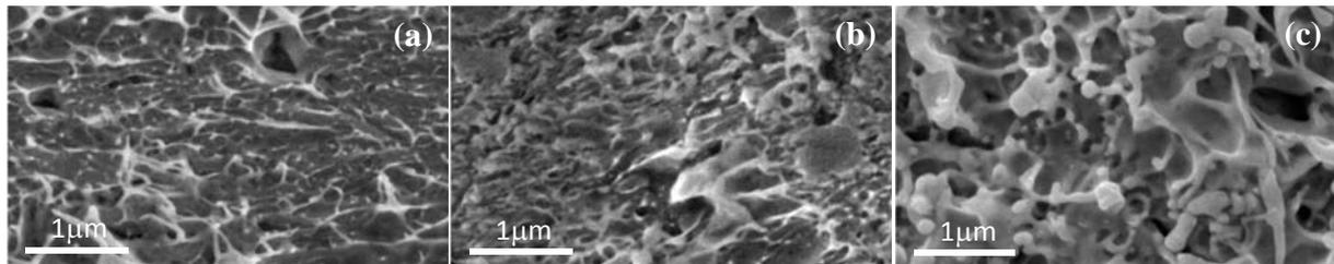
**Figure 6.** Enlarging of structures on gold with number of pulses  $N$ . (a)  $N = 1$ , (b)  $N = 5$ , (c)  $N = 20$ . High frequency soft X-ray oscillations do not excite plasmons. Outwardly structures are similar to that obtained in MD simulations, compare figures 4 and 6.
