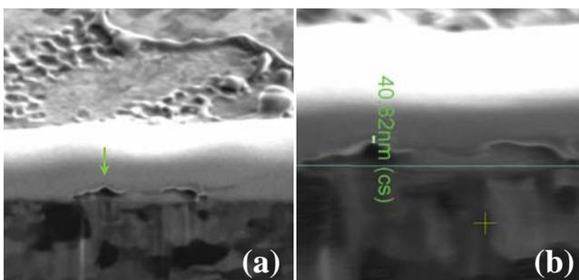
**Figure 5.** Focused ion beam (FIB) analysis unveils two bubbles frozen into solid Ta under surface. The left bubble is marked by the arrow in a general view (a). Thickness of the tantalum cover located above a bubble is measured in an enlarged picture (b). Height of the left bubble is  $186 \text{ nm}$ . The blue straight in (b) marks average surface.
